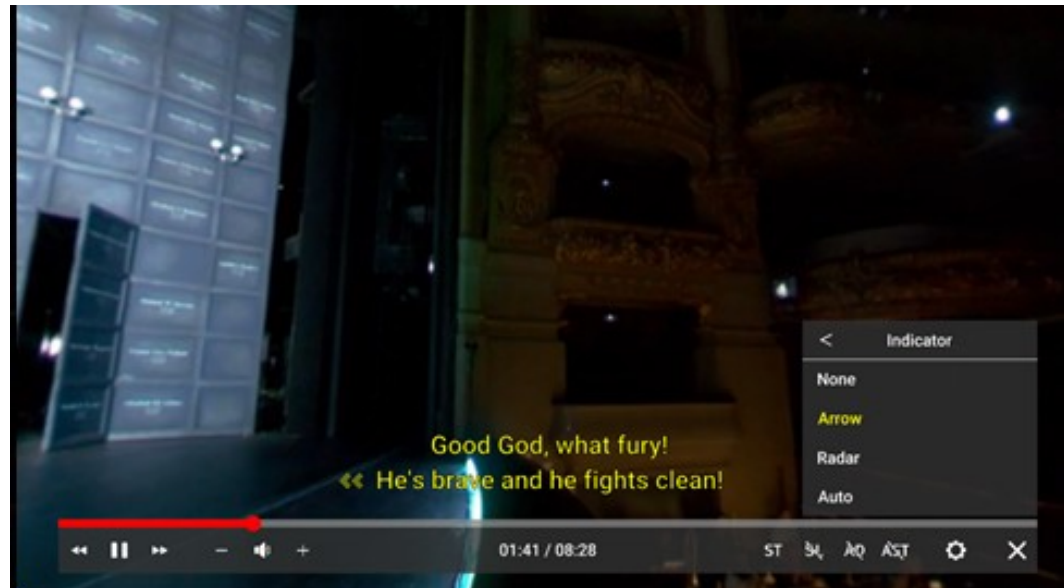
Figure 5: Subtitles with arrows (with intermittence effect) as a guiding method. When this position is inside the user's Field of View, the arrows are hidden. Likewise, an intermittence effect can be added to the arrows to catch the attention of the user.
