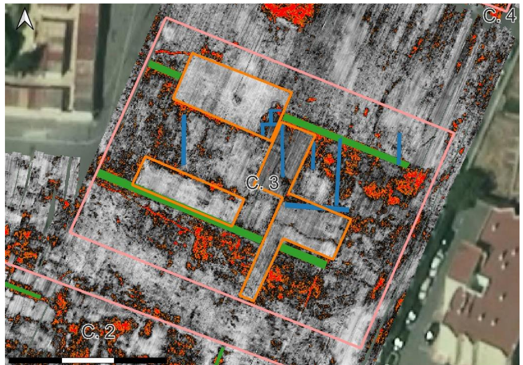
Figure 7. Detail of Set 3 in the central part of the study area showing (orange) the alterations of the subsoil by recent actions.
