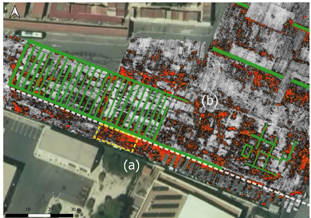
Figure 6. (a) Detail of Set 1 at the S end of the study area where the radargram signal is located (yellow dashed line) (Figure 5). (b) Detail of Set 2 where the main alignments are highlighted (green).
