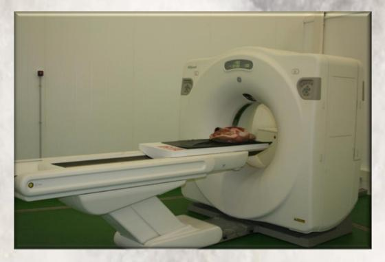
Salt and water contents can be estimated non-destructively by Computed Tomography (CT), which permits the monitoring of the same product during all the processing.
