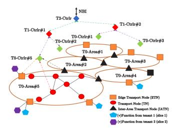
Figure 5. 5G-XHaul Control Plane architecture.
