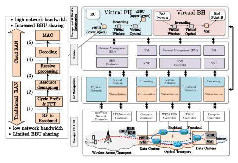
Figure 1. The overarching architecture supporting functional split processing [7].
