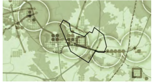
FIGURE 7. Excerpt from the SDRIF that shows priority densification areas from a regional perspective (big dots). These are mainly situated around suburban train stations (large white circles). Architects and planners working for suburban municipalities in the Paris Region use this guidance plan as a starting point for an in-depth morphological analysis of the urban fabric and of its evolution potential. Source: SDRIF (2013)
