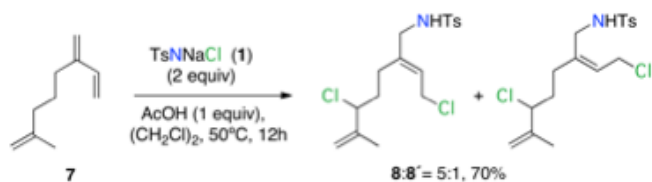
Scheme 6. Triple C-H oxidation of myrcene (7) with the 1/HOAc reagent combination.
